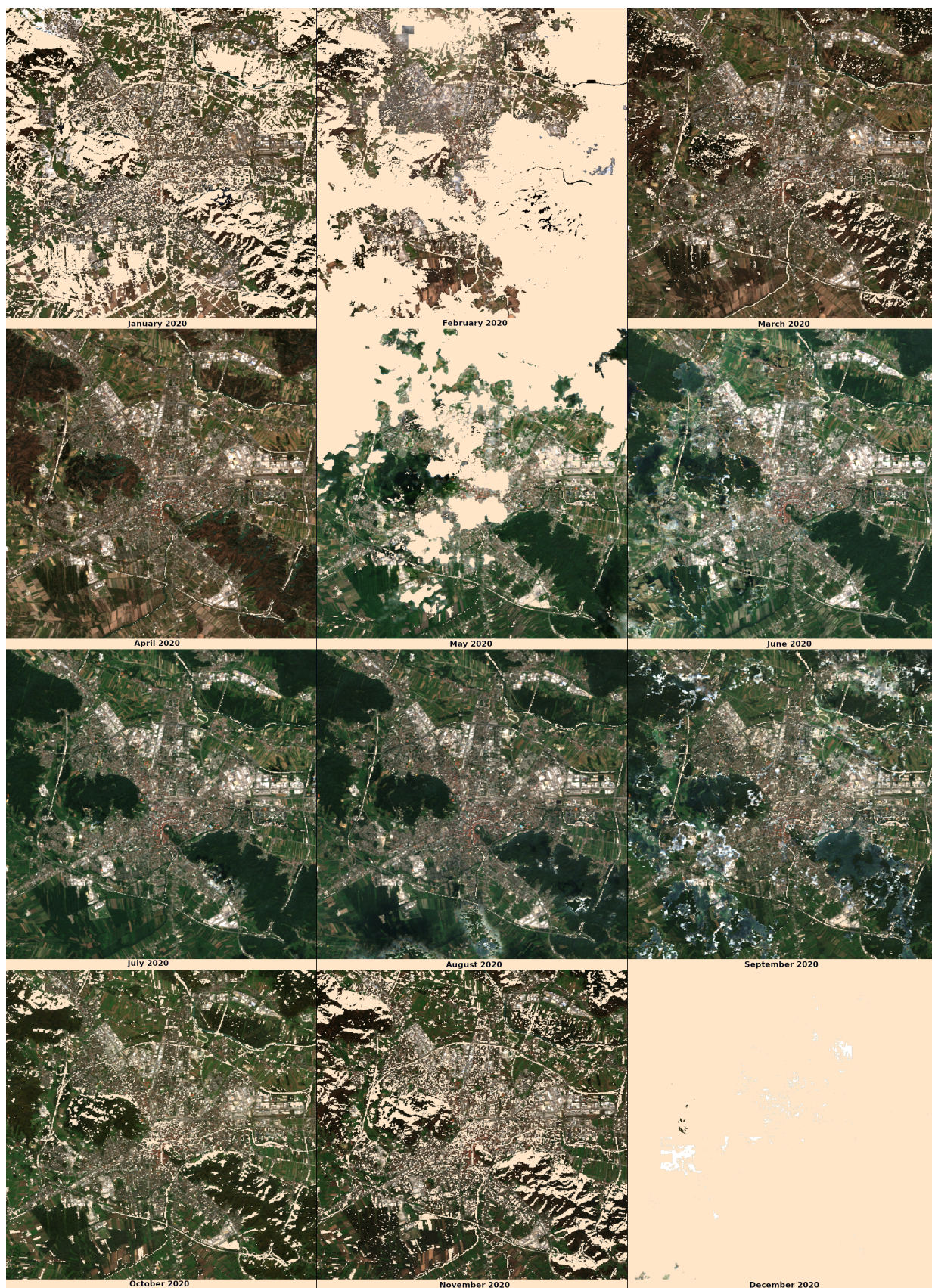
Figure D.2 – Visualization of monthly natural color imagery (using bands B04, B03 and B02) for Ljubljana (subset=Lat(46.005356:46.108536), Lon(14.431717:14.579785)) throughout 2020, with filter=SCL in (4,5,6) (vegetation, bare soils and water)
